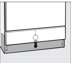
The emergency release cord is located at the bottom of the machine behind the service panel. Pull it downwards to open the door.
