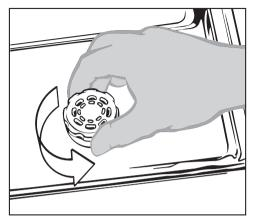
■ Undo the screw cap.
