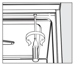
Secure the machine to the front edge of the worktop using screws through the holes on the left and right hand sides of the front trim.
