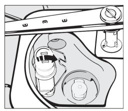
Lift up the non-return valve and rinse under running water.
