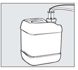
Place the container on the floor next to the washer-disinfector or in an adjoining cupboard.
